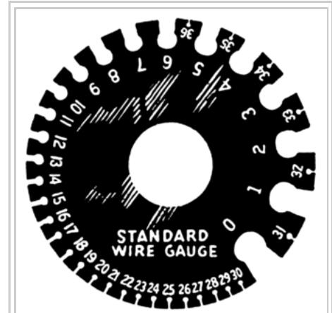
A device for measuring standard wire gauge.
