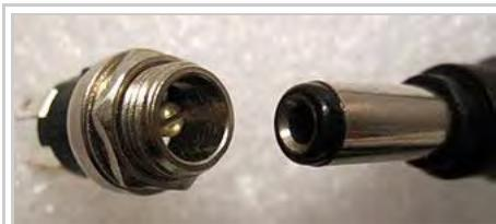
Common 5.5×2.5 mm coaxial power connectors. Power is provided by the *female plug* on the right to the *male jack* on the left; the exposed conductors are not hazardous due to the low voltage. See text for further explanation.
