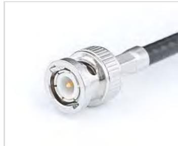
A *male* 50 ohm BNC connector *plug*. Three circular projections (including the central pin) interlock with two rings of the female jack.
