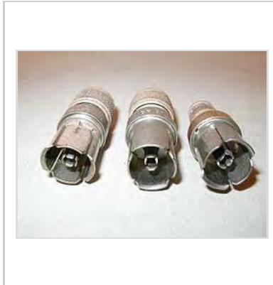
General Radio GR-874 hermaphrodite coaxial RF connector
