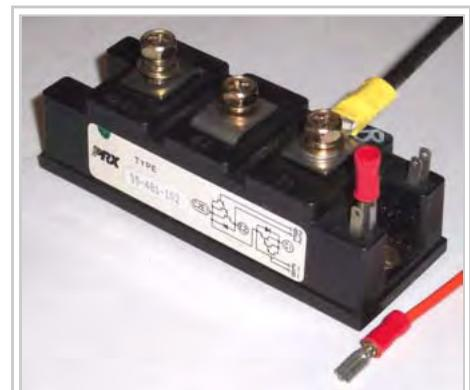
High-power transistor switch module with large screw connectors and small crimped-on "Fast-on" connectors
