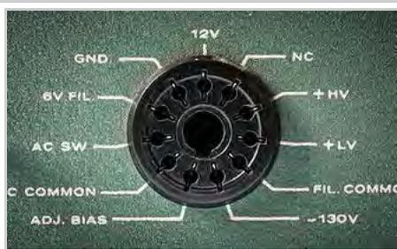
Heathkit power supply female connector for tube equipment
