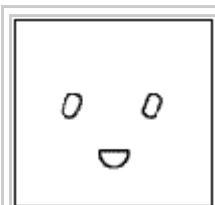
Socket for the tilted flattened pins and half-round earth pin of Danish computer equipment plug (mainly used in professional environment), standard DK 2-5a
