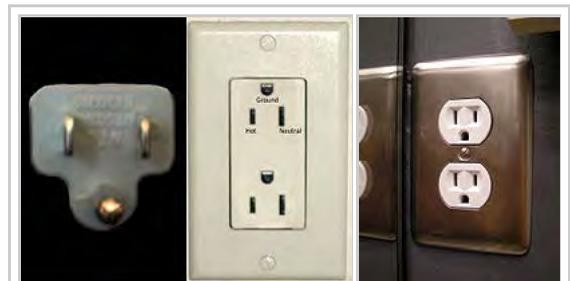
NEMA 5-15 plug, left. Decorative-style duplex socket, with orientation as specified in NECA 130-2010, center. Ordinary duplex socket, with orientation typically found, right. Photos are different scale—parallel blades are on 1/2 inch (12.7 mm) centers.
