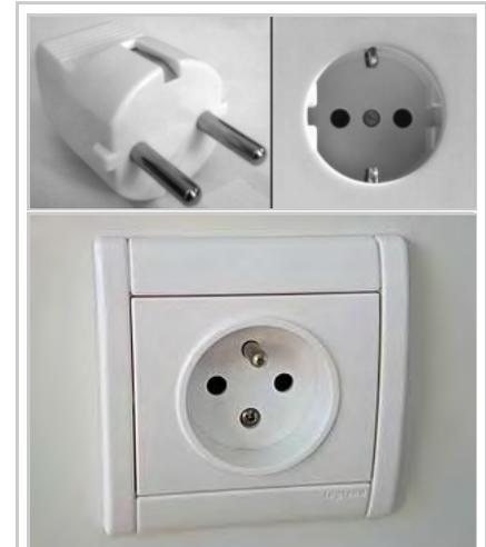
Plugs and sockets may sometimes combine male and female contacts, but the exposed pins or terminals in the socket are not energized. Clockwise from top left: CEE 7/4 (German) plug and matching CEE 7/3 socket; CEE 7/5 (French) socket.
