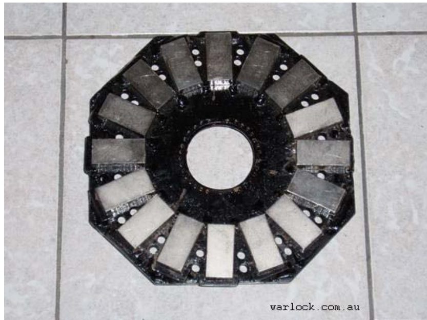
Figure 4. Front half of generator rotor with magnets attached
