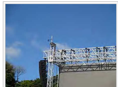
Anemometer on an outdoor stage set, to measure wind speed
