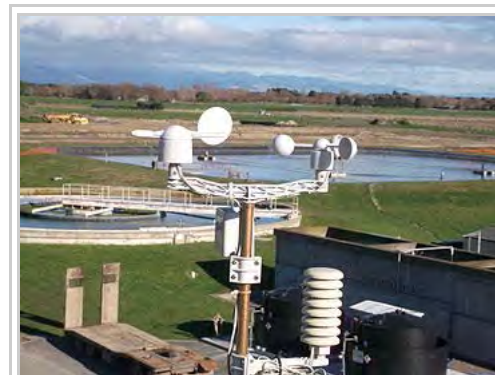
An anemometer is commonly used to measure wind speed.
