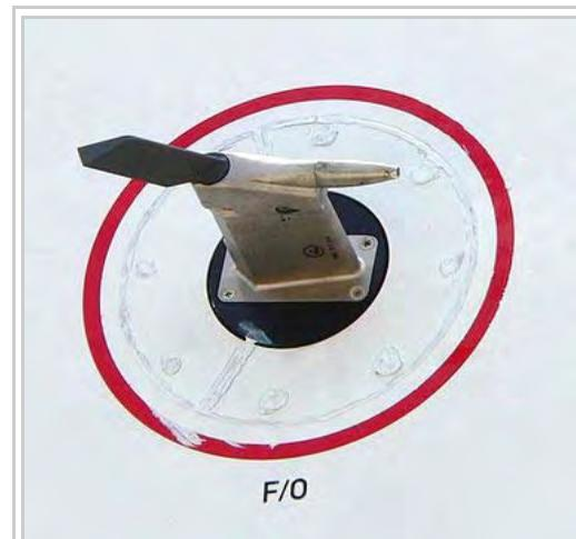
Aircraft use pitot tubes to measure airspeed. The example, from an Airbus A380, combines a pitot tube (right) with a static port and an angle-of-attack vane (left). Air-flow is right to left.
