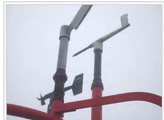
Weather instruments at Mount Washington Observatory. Pitot tube static anemometer is on the right.
