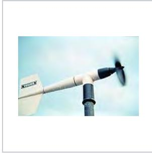
Vane style of anemometer
