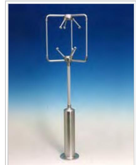
3D ultrasonic anemometer
