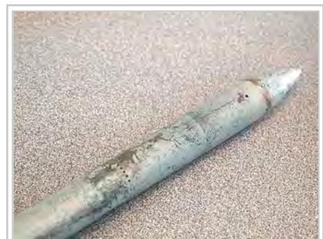
The pointed head is the pitot port. The small holes are connected to the static port.
