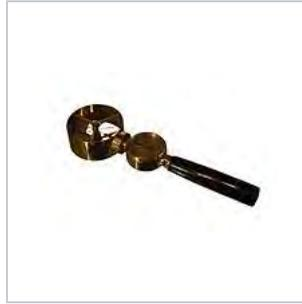
Hand-held low-speed vane anemometer
