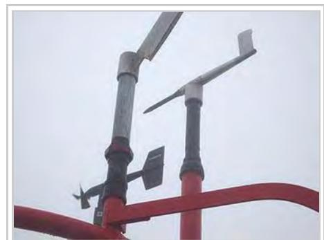
Instruments at Mount Washington Observatory. The pitot tube static anemometer is on the right.
