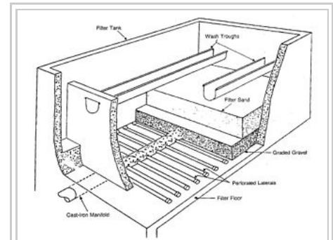
Cutaway view of a typical rapid sand filter
