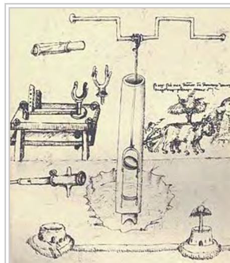
First European depiction of a piston pump, by Taccola, c.1450. [12]
