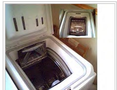
European top loader with horizontal axis rotating drum (2008)
