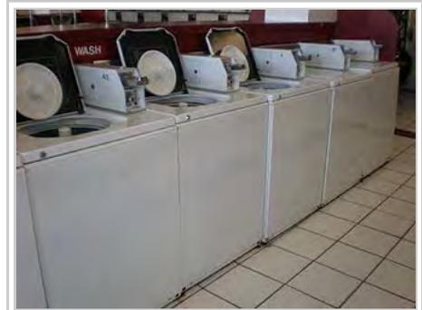
General Electric Filter-Flo top loading, vertical axis machines in laundromat. The pans on the inside of the lid are placed atop the agitator, and wash water is pumped through the perforated pans to collect lint. (California)
