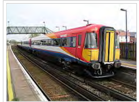
A passenger train, taking power through a third rail with return through the traction rails
