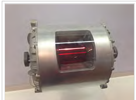
Cutaway view of a Tesla Model S drive motor
