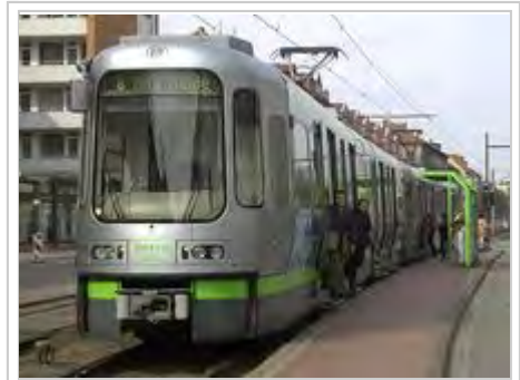
A streetcar (or Tram) drawing current from a single overhead wire through a pantograph.
