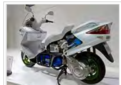
Suzuki Burgman (fuel cell prototype)
