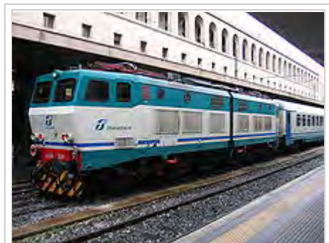
FS Class E656, an articulated Bo'-Bo'-Bo' locomotive, manages more easily the tight curves often found on the Italian railways
