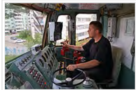
The operating controls of VL80R freight locomotive from Russian Railways. The wheel controls motor power.
