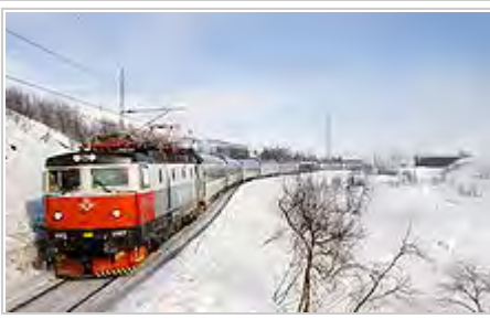
The Swedish Rc locomotive was the first series locomotive that used thyristors with DC motors.
