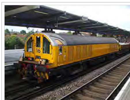
A London Underground battery-electric locomotive at West Ham station used for hauling engineers' trains
