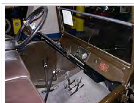
In the Ford Model T the left-side hand lever sets the rear wheel parking brakes and puts the transmission in neutral. The lever to the right controls the throttle. The lever on the left of the steering column is for ignition timing. The left foot pedal changes the two forward gears while the centre pedal controls reverse. The right pedal is the brake.
