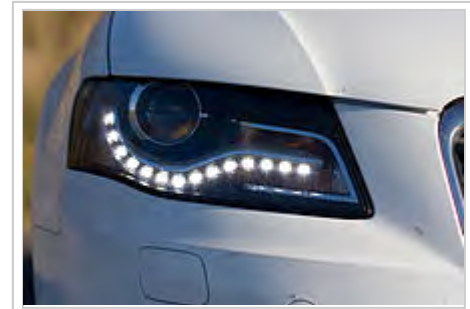
LED daytime running lights on an Audi A4
