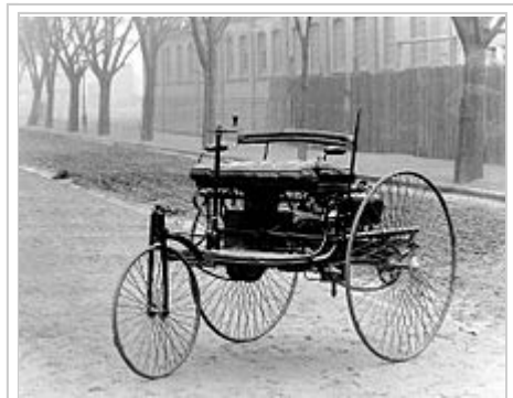
A photograph of the original Benz Patent-Motorwagen, first built in 1885 and awarded the patent for the concept
