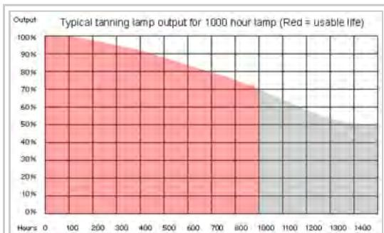
Typical output curve of a 1,000-hour-rated low-pressure tanning lamp. At 1,000 hours, the output becomes less than 70% of rated power.
