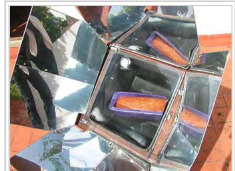
Solar stove used for cooking dishes [23]
