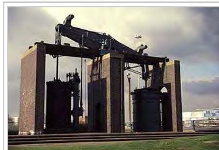
An 1817 Boulton & Watt beam blowing engine, used in Netherton at the ironworks of M W Grazebrook. Re-erected on the A38(M) in Birmingham, UK
