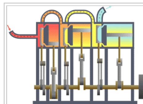
An animation of a simplified triple-expansion engine. High-pressure steam (red) enters from the boiler and passes through the engine, exhausting as low-pressure steam (blue), usually to a condenser.
