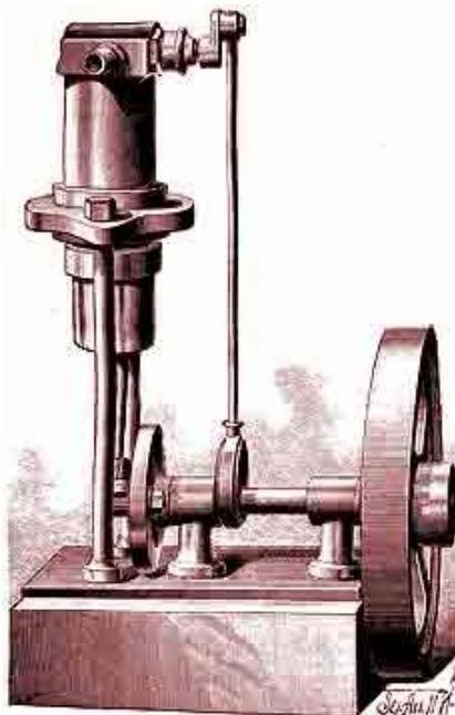
The cylinder and piston are made from mandrel drawn brass tubing, which may be purchased in any desired quantity in New York city. The fittings are mostly of brass, that being an easy metal to work.
