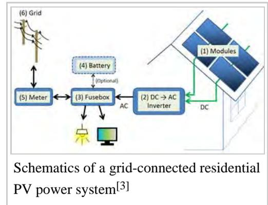
Many residential PV systems are connected to the grid wherever available, especially in developed countries with large markets.<sup>[9]</sup> In these grid-connected PV systems, use of energy storage is optional. In certain applications such as satellites, lighthouses, or in developing countries, batteries or additional power generators are often added as back-ups. Such stand-alone power systems permit operations at night and at other times of limited sunlight.
