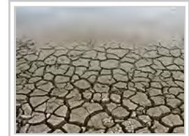
Shrinkage caused by drying
