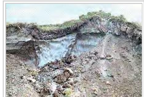
Slope failure of permafrost soil, revealing ice lenses.
