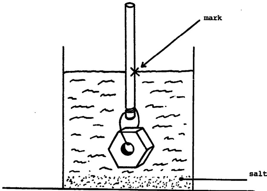
Fig. 1 The gauging of the stick or tube
