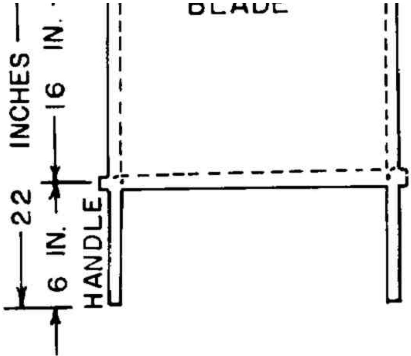
To make a durable 2-handled fan, first make its frame out of 2 sticks each 14 inches long and 2 sticks each 22 inches long. See sketch. To strengthen the corners, overlap the sticks about one-half inch, as shown.
