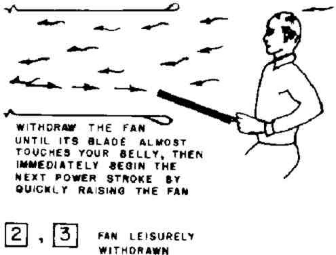
1) Quickly raise the fan to a vertical position close in front of your face and immediately fan (push) a slug of air into the opening - ending the power stroke with your arms fully extended and with the fan almost horizontal and out of the way of air that was "sucked" behind the fan and is still flowing out through the opening.
