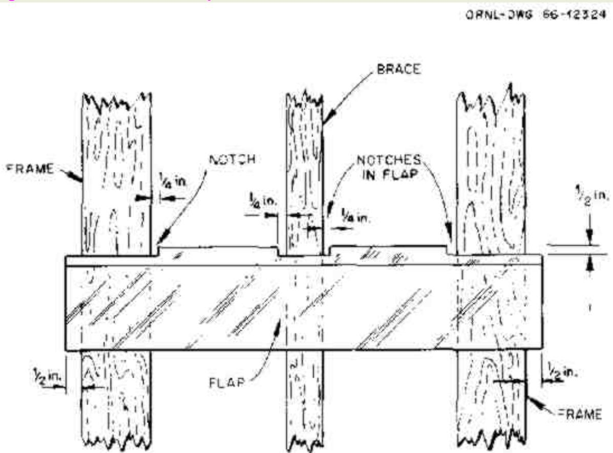
Fig. 6. Sizes of notches in flaps.
