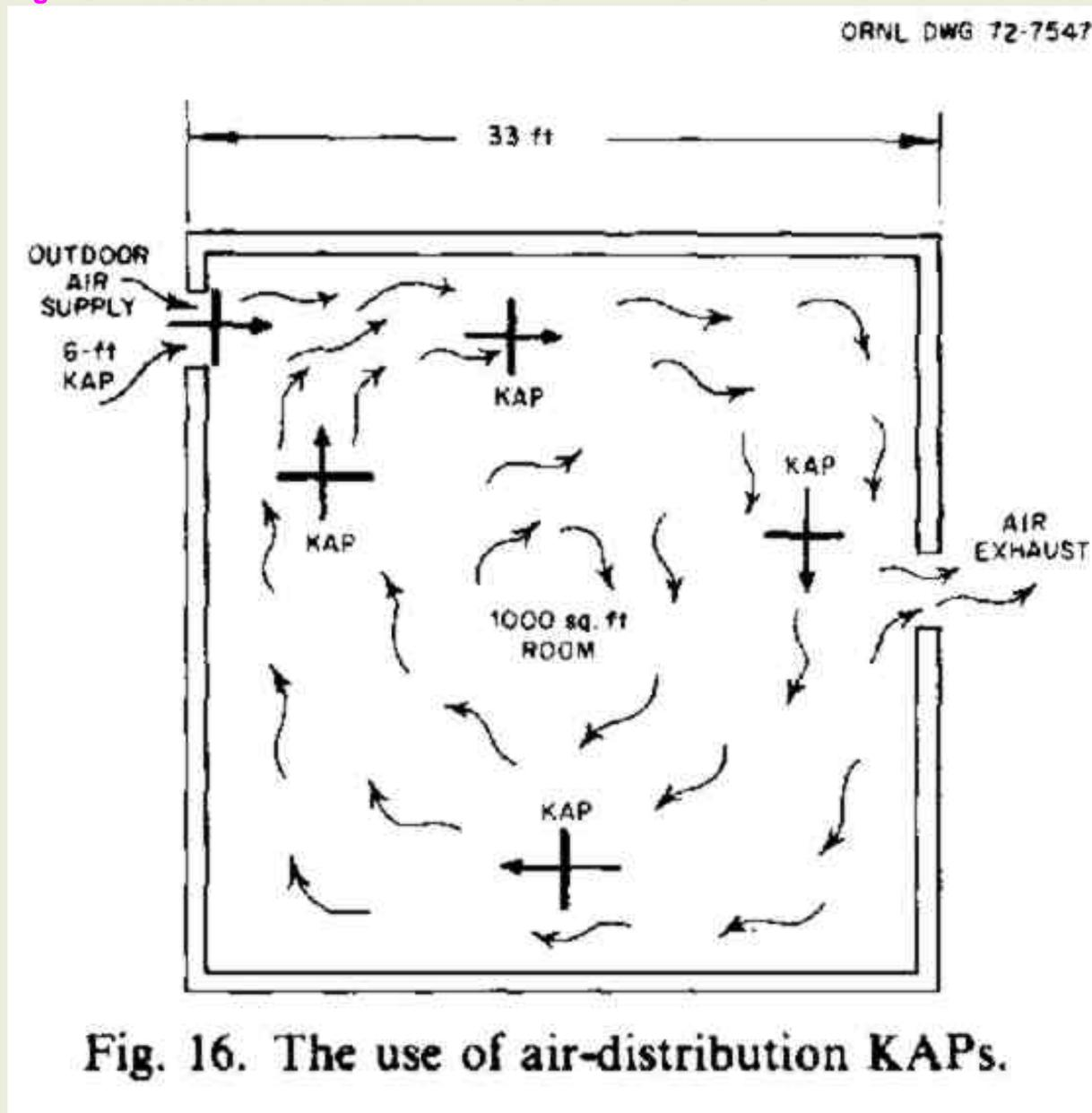
Fig. 16. The use of air-distribution KAPs.
