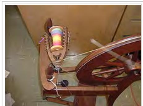
A single-drive wheel with the drive band around flyer and brake on the bobbin
