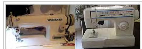
Industrial Sewing Machine (left), Domestic Sewing machine (right)
