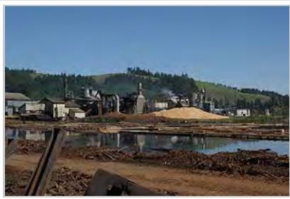
Oregon Mill using energy efficient ponding to move logs
