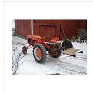
An Allis-Chalmers Model B with a saw mill style mechanism mounted on the back but normally used for cutting 4 foot long cordwood into shorter "stove length" pieces for wood burning and heating.
