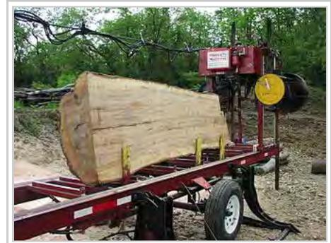
Bandsaw-Type Portable Sawmill
