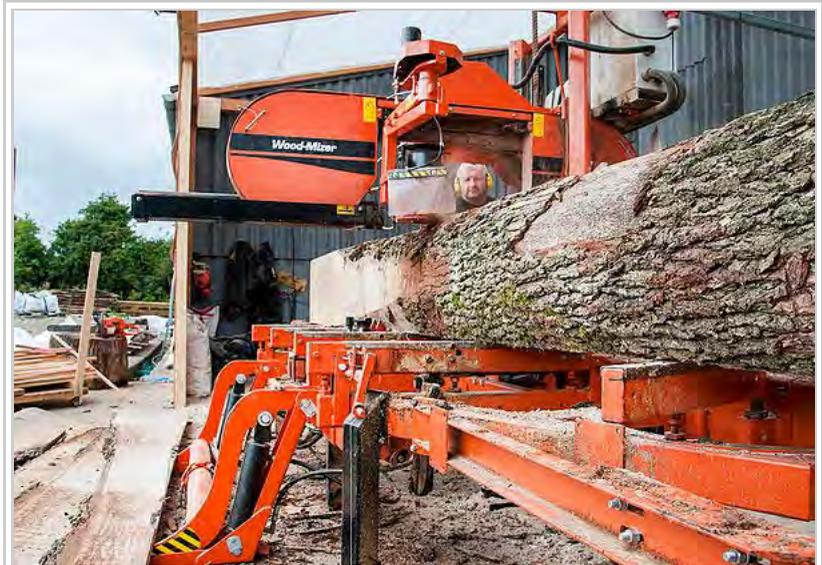
A portable sawmill enables small to medium-sized lumber producers the flexibility of cutting their own logs to their needs.
