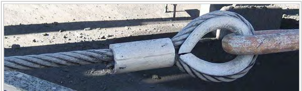
Right-hand ordinary lay (RHOL) wire rope terminated in a loop with a thimble and ferrule.
