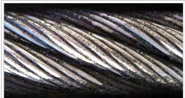
Right-hand Lang's lay (RHLL) wire rope (close-up). Right-hand lay strands are laid into a right-hand lay rope.
