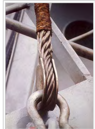
The ends of individual strands of this eye splice used aboard a cargo ship are served with natural fiber cord after the splicing is complete. This helps protect seaman's hands when handling.
