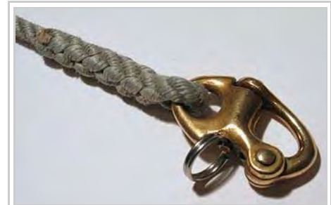
A line eye-spliced to a snap shackle.
