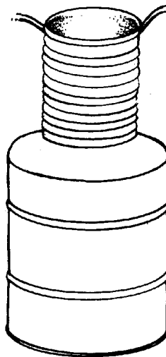
For a smaller cold storage space, wrap a 30-gallon drum with garden hose and insert it into a 55-gallon drum. Fill the space with insulation or very dry sawdust. Make a lid from styrofoam or other insulating material.
