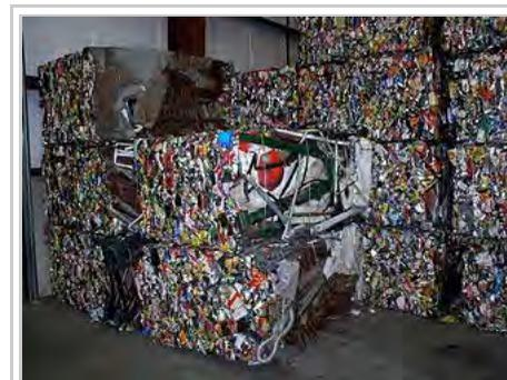
Steel crushed and baled for recycling
