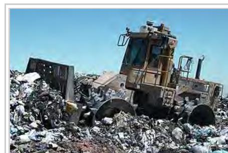
A landfill compaction vehicle in action.
