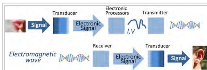
Radio communication. Information such as sound is converted by a transducer such as a microphone to an electrical signal, which modulates a radio wave sent from a transmitter. A receiver intercepts the radio wave and extracts the information-bearing electronic signal, which is converted back using another transducer such as a speaker.
