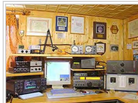
An example of an amateur radio station with four transceivers, amplifiers, and a computer for logging and for digital modes. On the wall are examples of various amateur radio awards, certificates, and a reception report card (QSL card) from a foreign amateur station.
