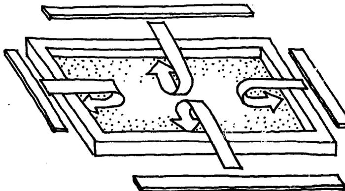
You are likely to find that after using the screen several times it becomes torn or clogs in places with dried ink or other wastes. When this happens you will have to take off the fabric and stretch new material onto the frame.
