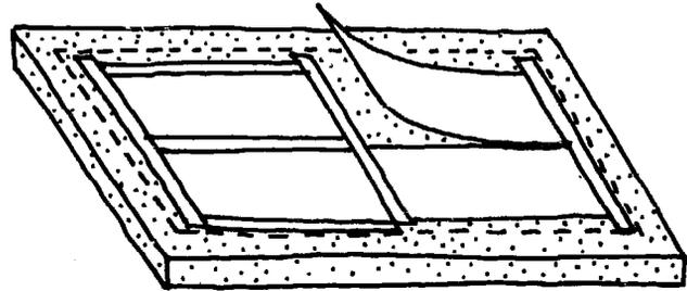
using either lots of gumstrip; or if you have a large area to cover, pieces of unused stencil stuck down with gumstrip. When you have completely masked the screen check that there are no holes where the ink can sneak through, by holding the screen up to the light. Cover any remaining holes with patches of gumstrip.
