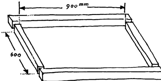
NB This drawing specifies internal dimensions in millimetres.
