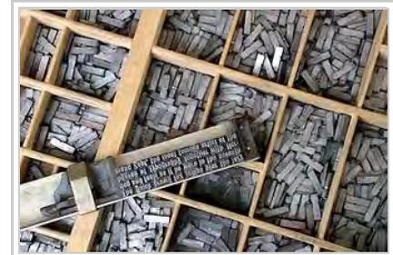
A case of cast metal type pieces and typeset matter in a composing stick
