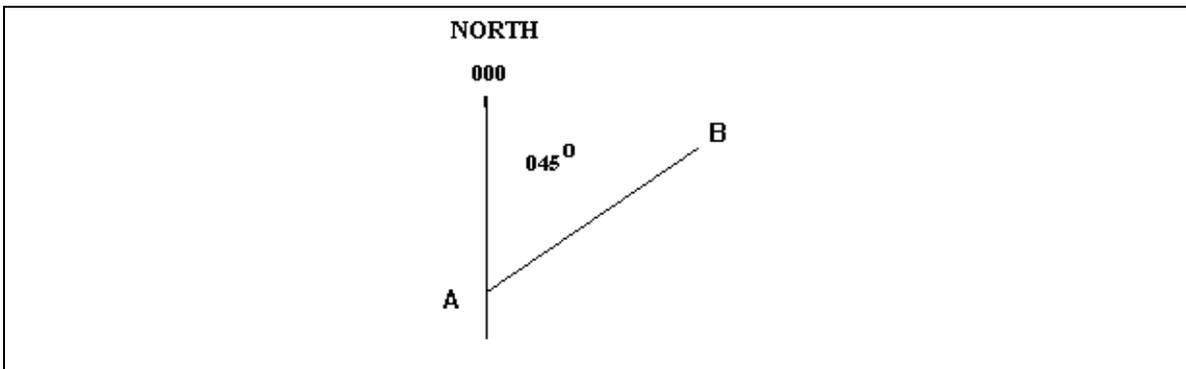
Figure 26 - Measuring bearings in degrees [A - B = 045 degrees]
