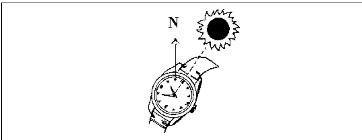
Figure 18 - direction-finding using a wrist watch
