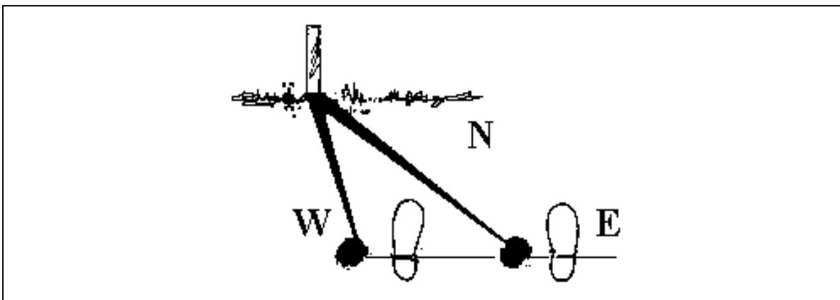
Figure 20 - The shadow stick method of direction finding
