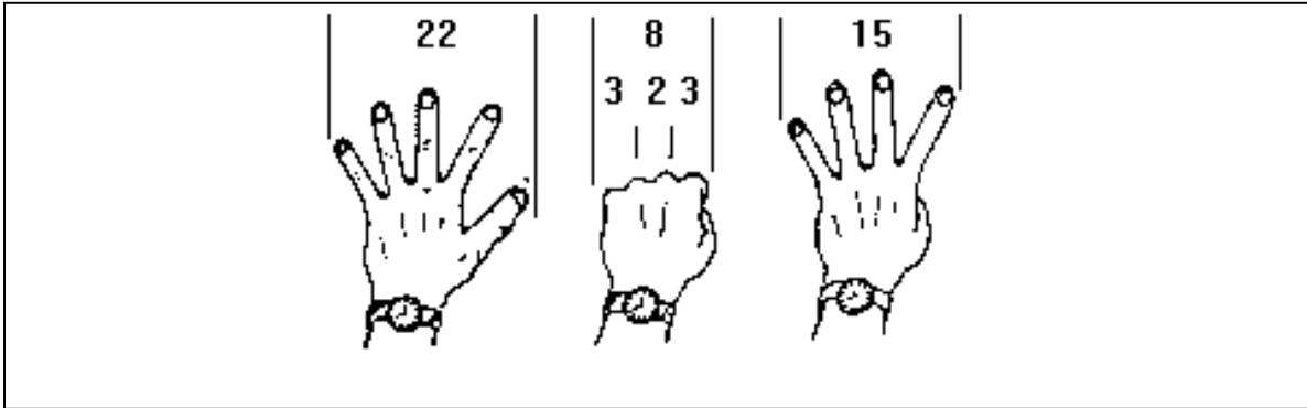
Figure 19 - The hand-span method of measuring sun movement
