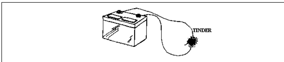
Figure 7 - The battery method of fire lighting
