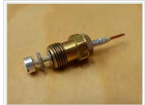
Thermocouple connection in gas appliances. The end ball (contact) on the left is insulated from the fitting by an insulating washer. The thermocouple line consists of copper wire, insulator and outer metal (usually copper) sheath which is also used as ground.<sup>[23]</sup>
