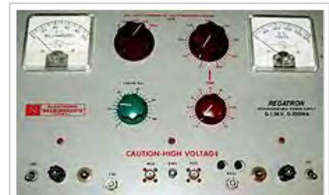
A rackmount, adjustable regulated DC power supply
