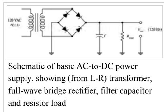
Schematic of basic AC-to-DC power supply, showing (from L-R) transformer, full-wave bridge rectifier, filter capacitor and resistor load
