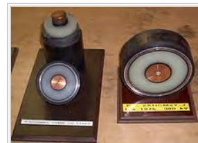
Segments of high-voltage cables
