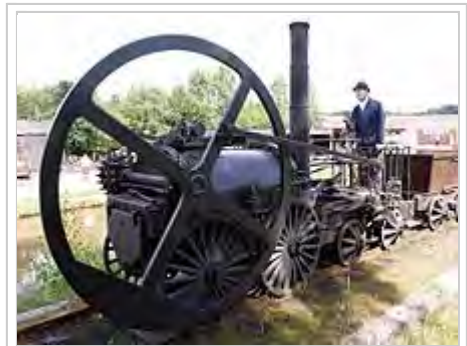
Trevithick's 1802 steam locomotive used a flywheel to even out the power of its single cylinder
