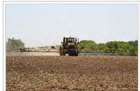
Large self-propelled agricultural 'floater' sprayer, engaged in pre-emergent pesticide application
