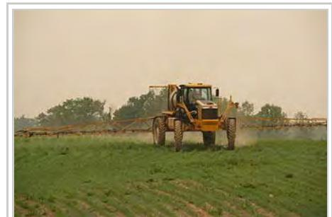
Self-propelled row-crop sprayer applying pesticide to post-emergent corn
