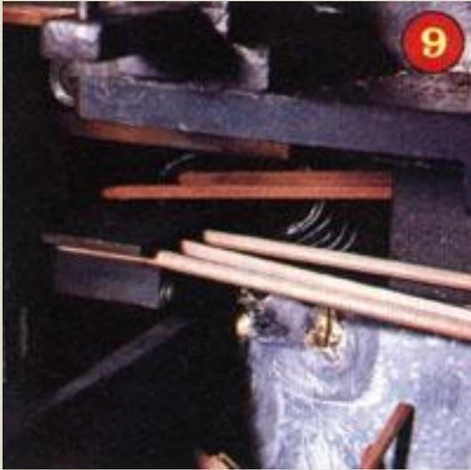
The same machine cuts apart each slat into eight separate pencils.
