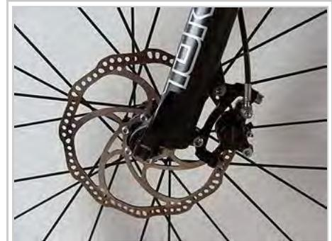
A front disc brake, mounted to the fork and hub
