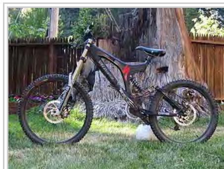
This is an upgraded entry level Downhill/Freeride bike: Specialized Bighit 2006 with 203 millimetres (8.0 in) of travel in the front and 190 millimetres (7.5 in) of travel in the back
