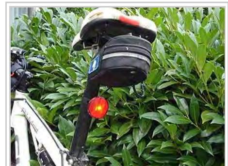
Home built "Red Giant" tail light. 1/2 W LED mounted in a standard reflector
