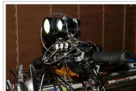
A homebrew HID light assembly consisting of a 10 watt HID light (right) and a 30 watt HID light (left) as well as three 1 watt Luxeon high power LEDs
