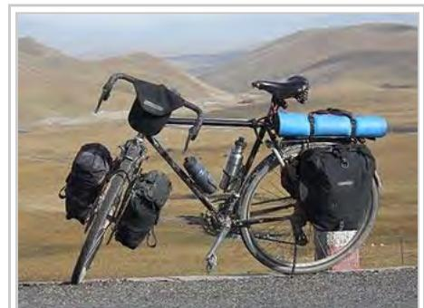
Touring bicycle equipped with front and rear racks, fenders/mud-guards, water bottles in cages, four panniers and a handlebar bag.
