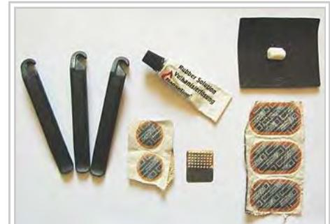
Puncture repair kit with tire levers, sandpaper to clean off an area of the inner tube around the puncture, a tube of rubber solution (vulcanizing fluid), round and oval patches, a metal grater and piece of chalk to make chalk powder (to dust over excess rubber solution). Kits often also include a wax crayon to mark the puncture location.
