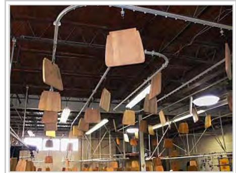
In this hangline approach, wood items being finished are moved through various finishing stages on a conveyor system
