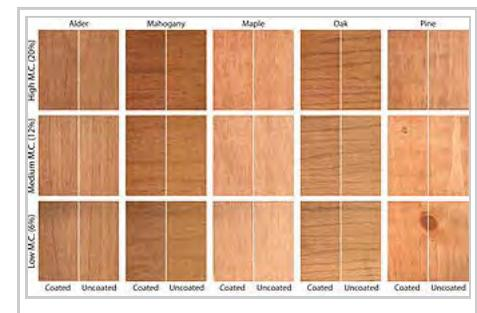
Wood's moisture content affects staining of wood.<sup>[15]</sup> Changes in wood moisture content can result in swelling and shrinkage of wood which can stress and crack coatings. Both problems can be avoided by stored wood indoors in an environment where it can equilibrate to a recommended moisture content (6 to 8%) that is similar to that of the intended end use of the furniture.<sup>[7]</sup>
