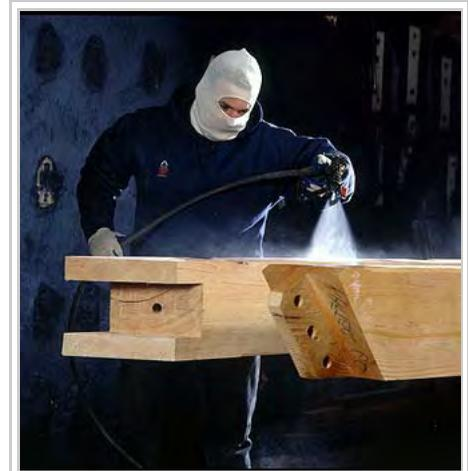
A worker sprays a urethane finish onto a timber
