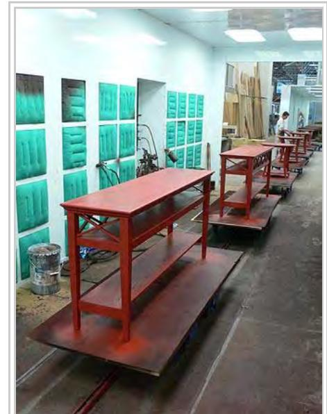
In this Towline method, mobile carts move large furniture through various finishing stages on a conveyor system.
