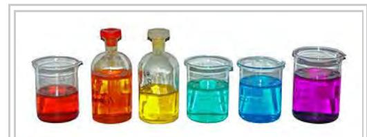
Transition metal compounds. From left to right, aqueous solutions of:  $\text{Co}(\text{NO}_3)_2$  (red);  $\text{K}_2\text{Cr}_2\text{O}_7$  (orange);  $\text{K}_2\text{CrO}_4$  (yellow);  $\text{NiCl}_2$  (turquoise);  $\text{CuSO}_4$  (blue);  $\text{KMnO}_4$  (purple).
